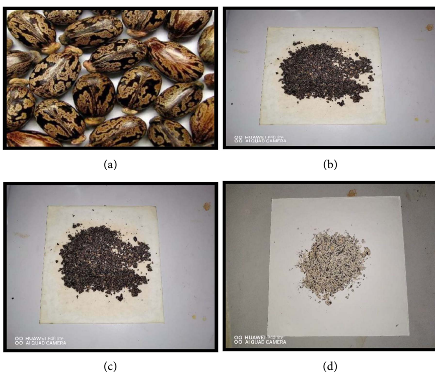
Figure 2. (a) The castor seed before being processed; (b) Crushed castor seeds before extraction and drying; (c) Crushed castor seed after drying before extraction; (d) Crushed castor seed after solvent extraction and drying.
