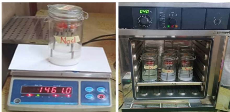
Figure 2. Ventilated desiccation oven for tomato slices/controlled temperature and humidity.
