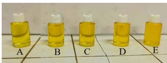
Figure 5. (A) Oil filtered on 5% activated carbon; (B) oil filtered with 3% activated carbon; (C) oil filtered on filter cloths; (D) oil filtered on dune sand; (E) crude oil from the seeds of the baobab fruit ( Adansonia digitata L.).
