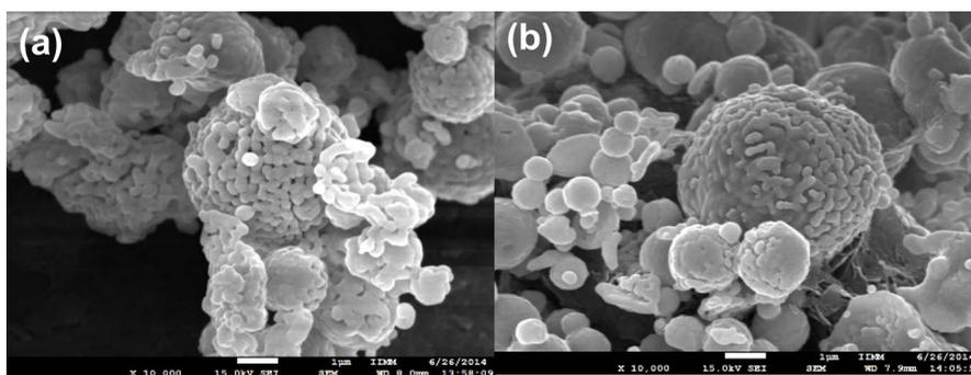
**Figure 2.** SEM micrographs of powders obtained at  $1600^\circ\text{C}$  of calcination temperature.
