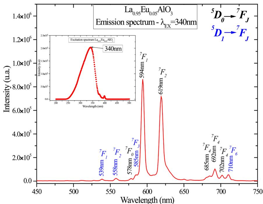
**Figure 4.** PL Emission spectra of  $\text{Eu}^{3+}$  5% doped  $\text{LaAlO}_3$  excited at 340 nm wavelength.
