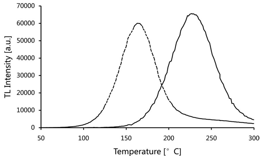
**Figure 5.** TL glow curve of: — LaAlO<sub>3</sub>:Eu<sup>3+</sup> powders (at UVR exposure). — LaAlO<sub>3</sub>:Eu<sup>3+</sup> induced by high energy X-ray beam.
