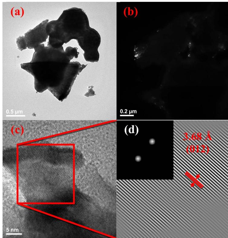
**Figure 3.** TEM micrographs of  $\text{LaAlO}_3:\text{Eu}^{3+}$  (5% Eu) powders synthesized at  $1600^\circ\text{C}$ : light field images in (a), dark field in (b), HRTEM image of  $\text{LaAlO}_3:\text{Eu}^{3+}$  (c) and HRTEM image (d) showing the plane (012) of rhombohedral phase.
