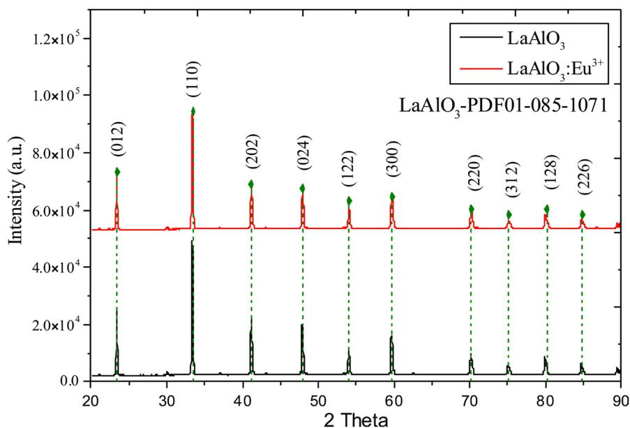
**Figure 1.** X-ray diffraction pattern of  $\text{LaAlO}_3:\text{Eu}^{3+}$  host lattice obtained at  $1600^\circ\text{C}$ .
