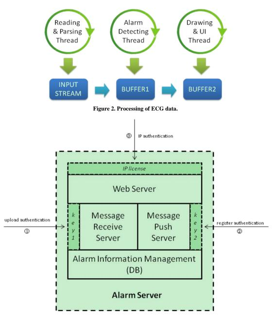
Figure 3. Alarm Server Architecture.
