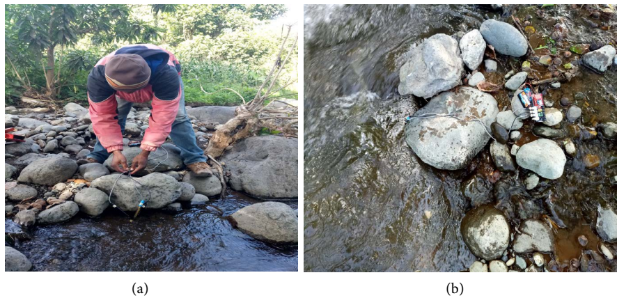
Figure 10. Testing of the developed prototype at Nduruma sub-catchment. (a) Installation of the WSN sensor node at the test site; (b) WSN sensor node taking measurements at the test site.
