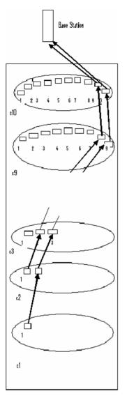
Figure 1. Transfer of data with the help of coordinators (Number 1 in every cluster is taken for CH, and all others  $(2, 3 \cdots 10)$  act as CCOs).
