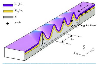
Figure 3. Schematic plot of the wrinkled pattern. Holes (solid circle) travel through a sinusoidal trajectory when a voltage is applied along (in x direction) the wrinkled pattern.
