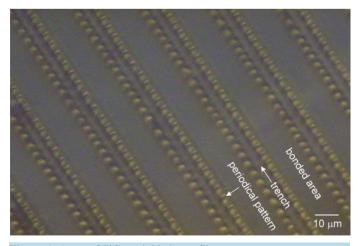
Figure 1. Array of SiGe wrinkled nanofilms.
