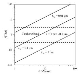
Figure 4. Emission spectra for different wrinkle periodicities. Dashed lines highlight the terahertz band.
