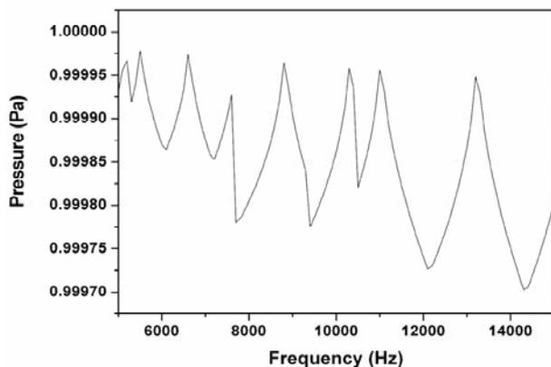
**Figure 2.** The pressure amplitude as function of frequency at distance 2 cm from the source.
