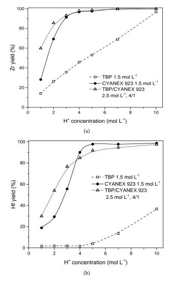
**Figure 4.** Efficiency in the extraction of Zr (a) and Hf (b) for the solvating extractants in nitric medium. Aqueous phase: 15.0 g·L<sup>-1</sup> of Zr, 0.6 g·L<sup>-1</sup> of Hf, 1.0 to 10.0 mol·L<sup>-1</sup> of H<sup>+</sup>, 1.3 to  $11 \text{mol·L}^{-1}$  of NO<sub>3</sub><sup>-</sup> and 25°C (±2).
