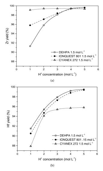
**Figure 2.** Efficiency in the extraction of Zr (a) and Hf (b) for the acid extractants in nitric medium. Aqueous phase: 15.0 g·L<sup>-1</sup> of Zr, 0.6 g·L<sup>-1</sup> of Hf, 1.0 to 5.0 mol·L<sup>-1</sup> of H<sup>+</sup>, 1.3 to 4.9 mol·L<sup>-1</sup> of NO<sup>3-</sup> and 25°C ( $\pm 2$ ).
