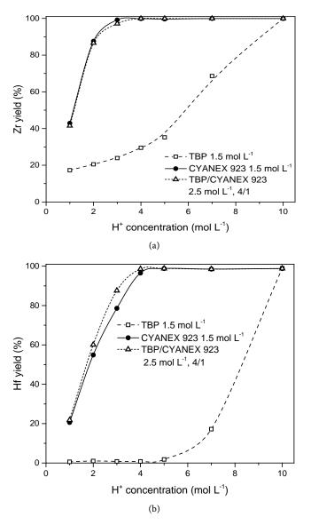
Figure 5. Efficiency in the extraction of Zr (a) and Hf (b) for the solvatingextractants in hydrochloric medium. Aqueous phase: 15.0 g·L<sup>-1</sup> of Zr, 0.6 g·L<sup>-1</sup> of Hf, 1.0 to 10.0 mol·L<sup>-1</sup> of H<sup>+</sup>, 1.1 to 10.8 mol·L<sup>-1</sup> of Cl<sup>-1</sup> and 25°C (±2).
