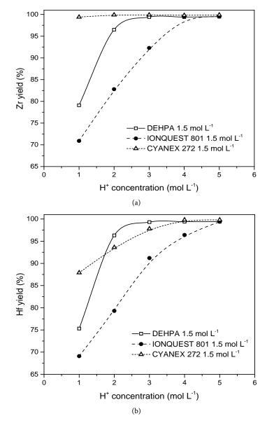
Figure 3. Efficiency in the extraction of Zr (a) and Hf (b) for the acid extractants in hydrochloric medium. Aqueous phase: 15.0 g·L^-1 of Zr, 0.6 g·L^-1 of Hf, 1.0 to 5.0 mol·L^-1 of H^+, 1.1 to 5.7  $mol \cdot L^{-1}$  of  $Cl^{-}$  and  $25^{\circ}C$  (±2).
