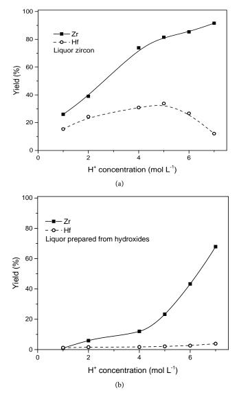
**Figure 6.** Efficiency in the extraction of Zr and Hf for zircon (a) and hydroxides (b) liquors. Aqueous phase: 15.0 g·L<sup>-1</sup> of Zr, 0.6 g·L<sup>-1</sup> of Hf, 1.0 to 7.0mol·L<sup>-1</sup> of H<sup>+</sup>, TBP 3.0mol·L<sup>-1</sup> and 25°C ( $\pm 2$ ).
