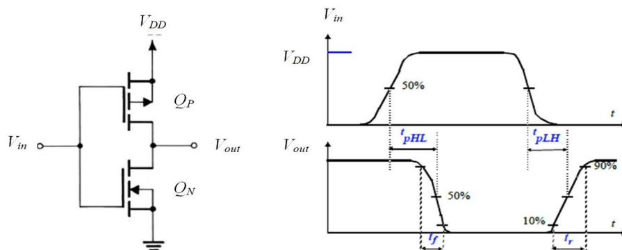
**Figure 1.** CMOS inverter performing the Boolean operation  $\bar{0} = 1$  and  $\bar{1} = 0$  (where  $1 = V_{DD}$ ). The time delays  $t_{pHL}$  and  $t_{pLH}$  brings about the notion that the switching is not instantaneous.
