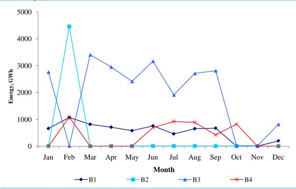
Figure 7. Green electricity sales in Finnish grid which include yearly purchase rate of 41 percent (5205 GWh/year, Scenario A2) for electricity import from Russia and Sweden: B1, B2, B3, B4 are electricity consumption of CHP plants, Households, Forest industry and electricity import, respectively.
