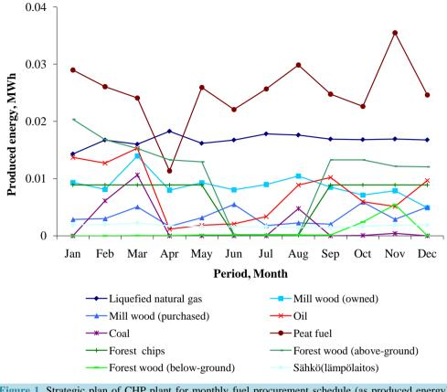
Figure 1. Strategic plan of CHP plant for monthly fuel procurement schedule (as produced energy), MWh/month [2].
