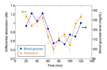
**Figure 6.** Changes in the differential absorption between 1152 and 1186 cm<sup>-1</sup> measured by the improved system. Changes in the blood-glucose level are also shown for comparison.
