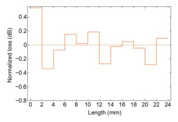
**Figure 4.** Losses measured when the upper surface of the prism is partially masked by an absorber after applying improvements.
