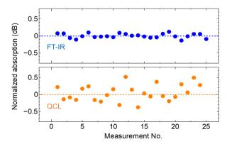
**Figure 2.** Measurement errors in the differential absorption between 1152 and 1186 cm<sup>-1</sup> for the FT-IR and QCL systems.
