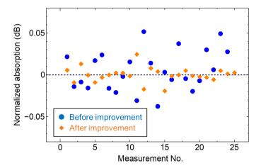
**Figure 5.** Differential absorption between 1152 and 1186 cm<sup>-1</sup> for 25 consecutive lip measurements using the original and improved systems.
