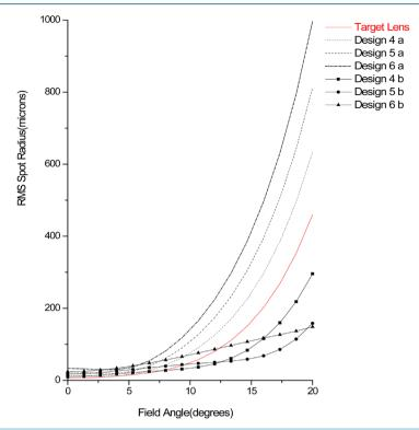
Figure 3. Comparison between the corresponding values of RMS Spot Radius for the target lens and the mid GRIN triplet design as function of field angles.
