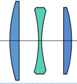
Figure 1. Scheme of a Cooke triplet lens.
