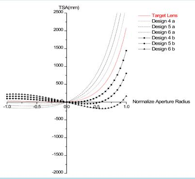
Figure 6. Comparison between the corresponding values of TSA for the target lens and the mid GRIN triplet as function of aperture radius at field angle  $= 20^{\circ}$ .
