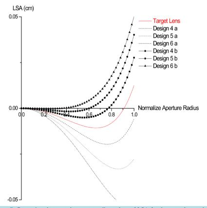
**Figure 7.** Comparison between the corresponding values of LSA for the target lens and the mid GRIN triplet design as function of upper half of the aperture radius for zero field angle.
