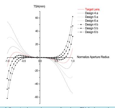
Figure 5. Comparison between the corresponding values o TSA for the target lens and the mid GRIN triplet design as function of aperture radius at zero field angle.
