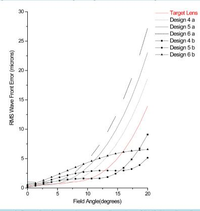
Figure 4. Comparison between the corresponding values of RMS Wave Front Error for the target lens and the mid GRIN triplet design as function of field angles.
