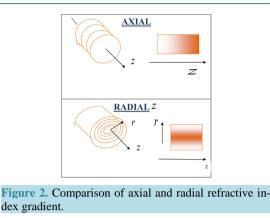
In lens design, the axial gradient-index lens has two important advantages. First, the curved lens surfaces still, focusing performance is far deviations. Second, axial gradient-index material can theoretically be fabricated in any size or thickness.
