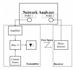
Figure 2. The experimental setup of VLC system.
