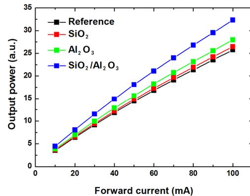
**Figure 7.** The output power characteristics of the non-passivated, the  $\text{SiO}_2$ -passivated, the  $\text{Al}_2\text{O}_3$ -passivated, and the  $\text{Al}_2\text{O}_3/\text{SiO}_2$ -passivated LED. The output power of the  $\text{Al}_2\text{O}_3/\text{SiO}_2$ -passivated LED exhibits about 25% higher than that of the non-passivated LED.
