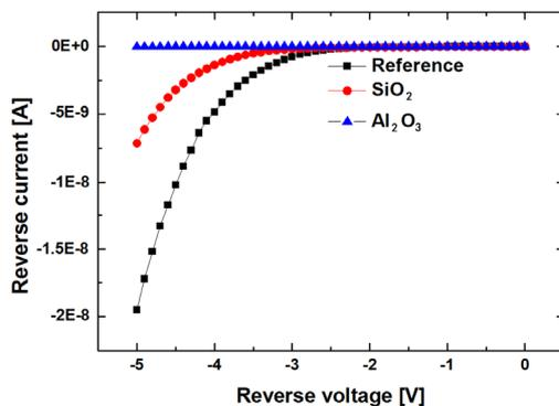
**Figure 6.** The LED with  $\text{Al}_2\text{O}_3$  layer exhibits at least two and three orders lower in leakage current compared to that with  $\text{SiO}_2$  layer and without dielectric layer, respectively.
