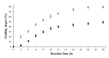
**Figure 6.** Grafting degree as function of reaction time, at constant temperature (60°C), styrene concentration 60/40 (V/V) in ethanol, pH ~3.5 and dose 2 kGy.  $\blacksquare$ ) FEP grafted with styrene and  $\blacklozenge$ ) ETFE grafted with styrene.
