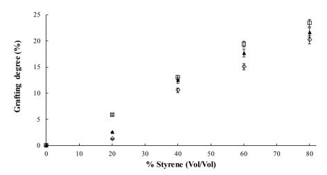
**Figure 1.** Grafting degree for ETFE as a function of the monomer concentration in ethanol at different dose, reaction temperature 60°C and reaction time 12 h.  $\diamondsuit$ ) 2 kGy,  $\blacktriangle$ ) 5 kGy and  $\square$ ) 10 kGy.
