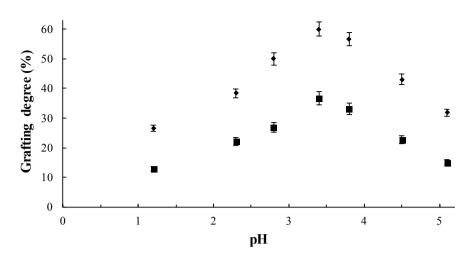
**Figure 4.** Grafting degree as a function of pH. Monomer concentration remained at 40% in ethanol, dose 2 kGy, reaction time 24 h, reaction temperature 70°C and pH was changed with  $H_2SO_4 0.05$  M.  $\blacklozenge$ ) ETFE and  $\blacksquare$ )FEP.
