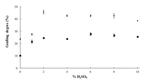
**Figure 3.** Grafting degree as a function of acid percentage added. Monomer concentration remained at 40% in ethanol,  $H_2SO_4$  0.05 M, dose 2 kGy, reaction temperature 70°C and reaction time 24 h  $\blacklozenge$ ) ETFE and  $\blacksquare$ )FEP.
