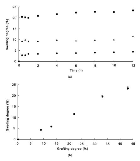
**Figure 9.** (a) Swelling degree as a function of time immersion in water. Sulfonated ETFE-g-St at different grafting degree: ●), 10% ▲) 22% and ■) 38 %; (b) Swelling degree as a function of grafting degree for ETFE-g-St.
