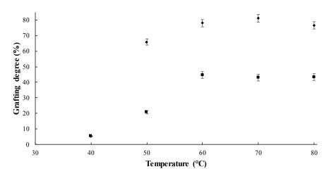
**Figure 5.** Grafting degree as a function of temperature. Dose 2 kGy, reaction time 24 h, pH ~3.5 and concentration (40/60 ethanol/styrene ■) FEP grafted with styrene and ◆) ETFE grafted with styrene.
