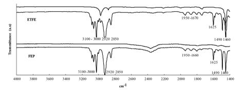
Figure 7. IR spectra of unmodified and modified ETFE and FEP with styrene.
