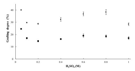
Figure 2. Grafting degree as a function of molar acid concentration 10% added in solution styrene/ethanol (40/50) at 2 kGy, reaction temperature 70°C and reaction time 24 h. ◆) ETFE and ■) FEP.
