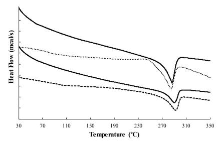
**Figure 8.** DSC thermograms of unmodified and modified fluoropolymers with styrene. ETFE-g-St and FEP-g-St.
