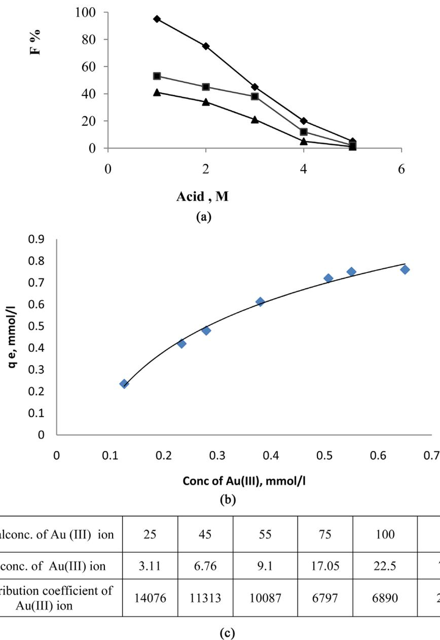
**Figure 1.** (a) Effect of acidity to the gold (III) sorption (•HCl, ■H<sub>2</sub>SO<sub>4</sub>, ▲HNO<sub>3</sub>); (b) effect of adsorbent dose; (c) calculated results of Au (III) distribution coefficient in solution.
