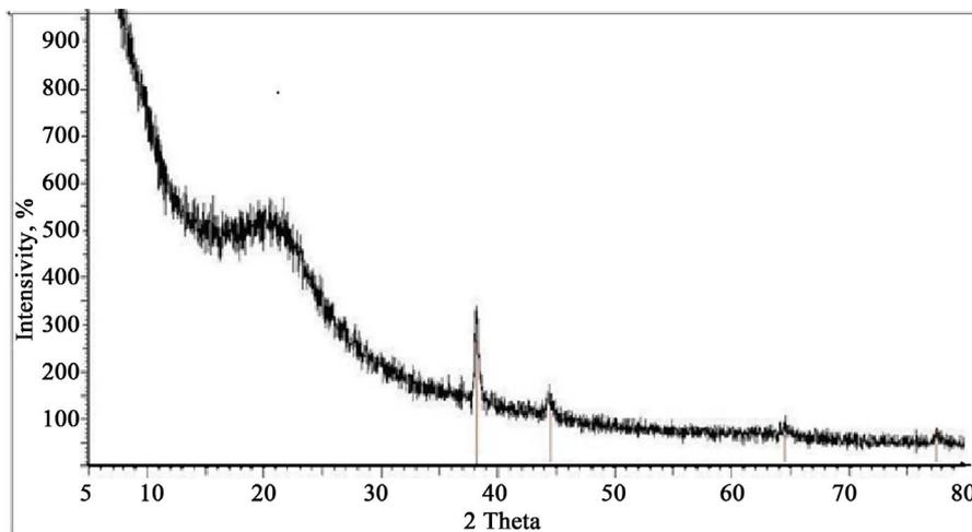
**Figure 2.** X-ray diffraction pattern of nanogold embedded polymer matrix.
