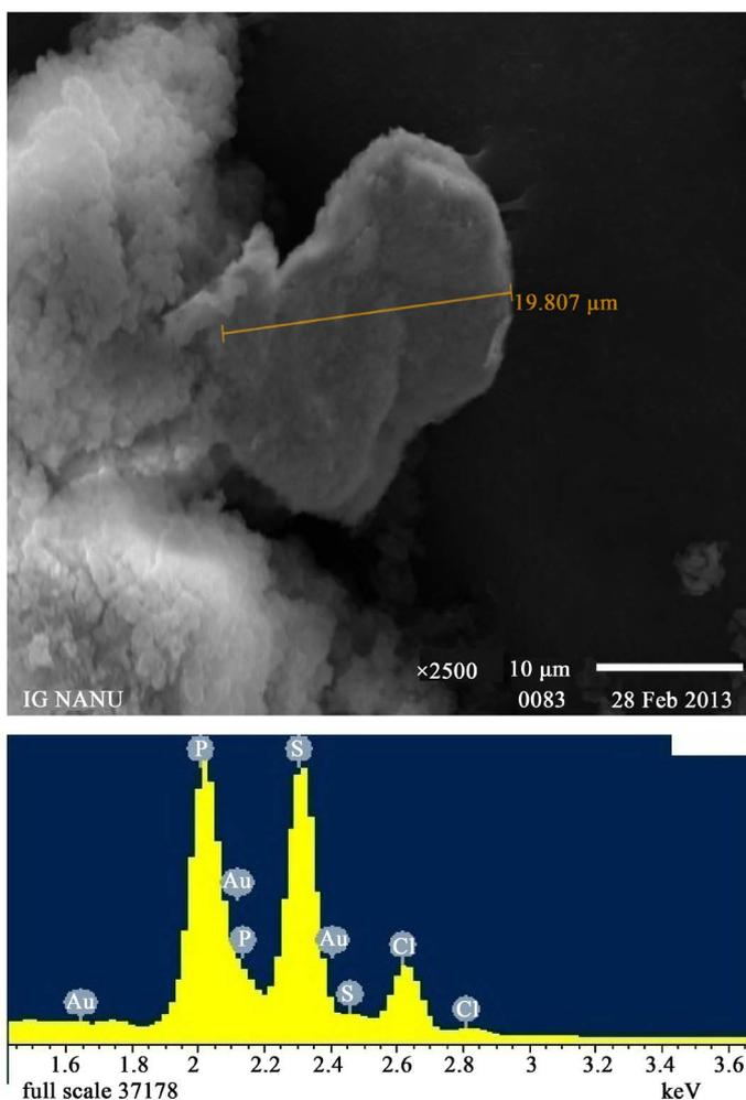
**Figure 3.** SEM image and EDS spectra of gold particles embedded polymer matrix.
