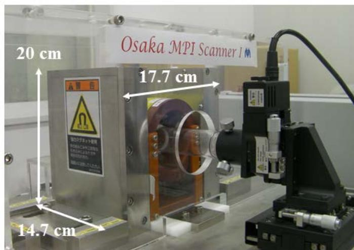
**Figure 1.** Photograph of our scanner for magnetic particle imaging (MPI).
