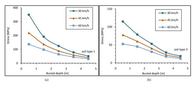
Figure 6. Maximum principal stresses in a 4-inch diameter steel pipe for different vehicle velocity.
