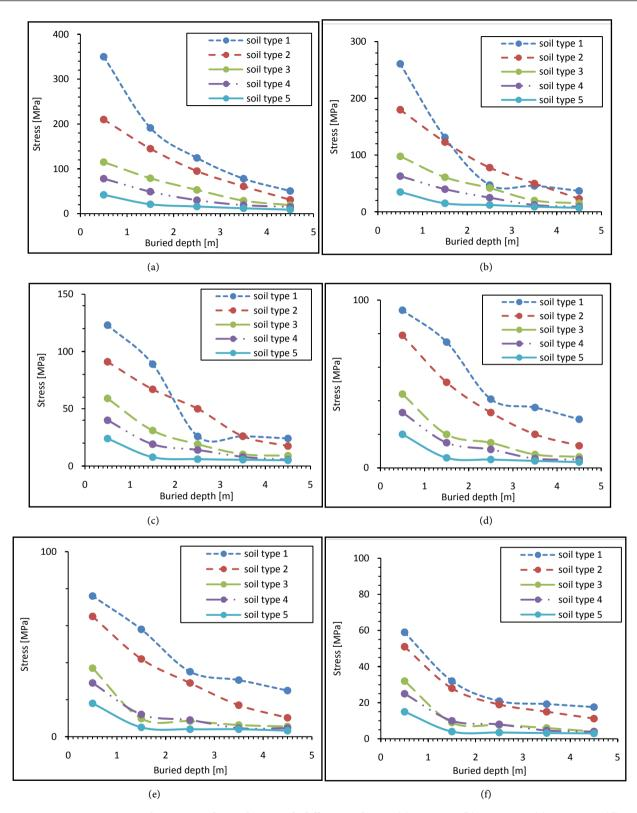
**Figure 10.** Maximum principal stresses in the steel pipe with different soil type. (a) D = 4 in; (b) D = 10 in; (c) D = 20 in; (d) D = 24 in; (e) D = 30 in; (f) D = 44 in.
