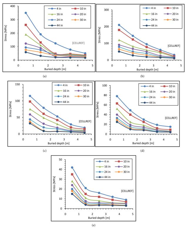
Figure 9. Maximum principal stresses in the steel pipe with different Diameter.
