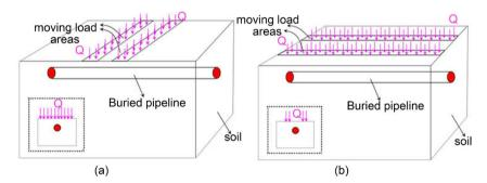
**Figure 1.** Schematic diagram of the buried pipeline under moving load. (a) Perpendicular motion; (b) Parallel motion.
