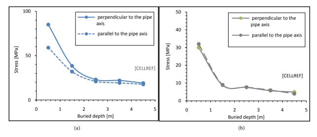
Figure 5. Maximum principal stresses in a 44-inch diameter steel pipe for different vehicle moving directions.
