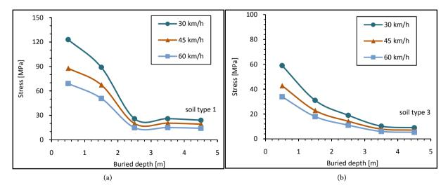
Figure 7. Maximum principal stresses in a 20-inch diameter steel pipe for different vehicle velocity.
