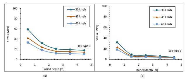
Figure 8. Maximum principal stresses in a 44-inch diameter steel pipe for different vehicle velocity.
