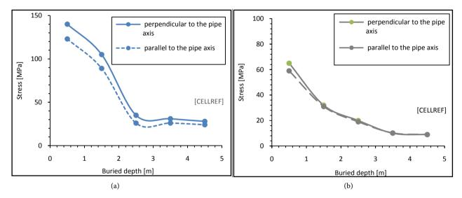
Figure 4. Maximum principal stresses in a 20-inch diameter steel pipe for different vehicle moving directions.
