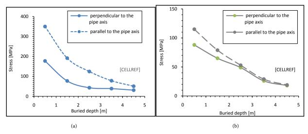
Figure 3. Maximum principal stresses in a 4-inch diameter steel pipe for different vehicle moving directions.
