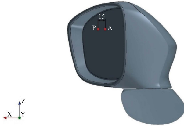
Figure 21. The measuring point P is located 15 mm away vertically over the measuring point A on the mirror surface.
