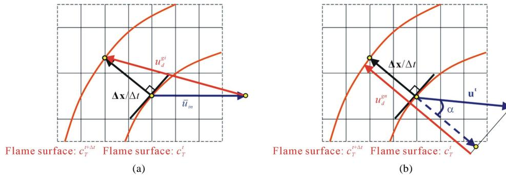
**Figure 2.** Schematic of simulating experimental analyses on the flame displacement speed. (a)  $u_d^{gi}$  obtained in consideration of the mean inflow velocity on the upstream boundary, (b)  $u_d^{gn}$  obtained in consideration of the normal component of the local flow velocity.
