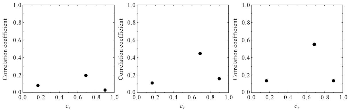
**Figure 8.** Correlation coefficients between non-dimensionalised  $u_d^{gn}$  and  $u_d^b$  on some isosurfaces of  $c_T$  with different Lewis numbers. From the left, case Ml, case Mm, and case Mh.
