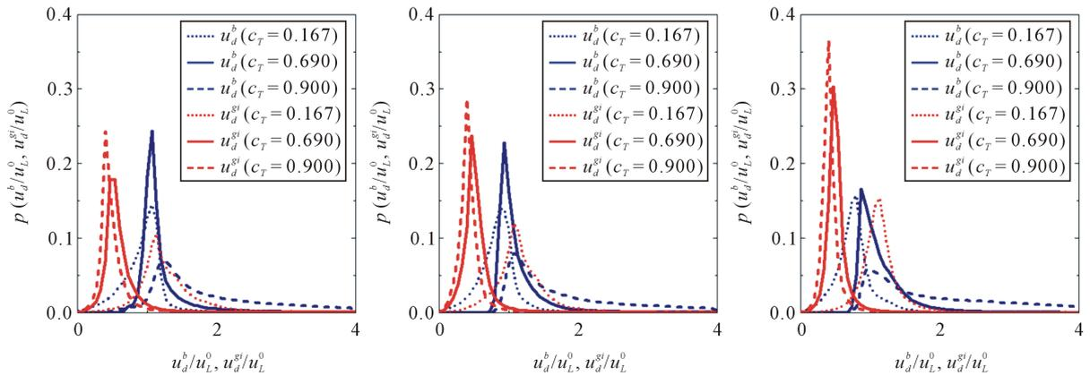
**Figure 3.** Probability density functions (pdfs) of non-dimensionalised  $u_d^{gi}$  and  $u_d^b$  on some isosurfaces of  $c_T$  with different Lewis numbers. From the left, case MI, case Mm, and case Mh.
