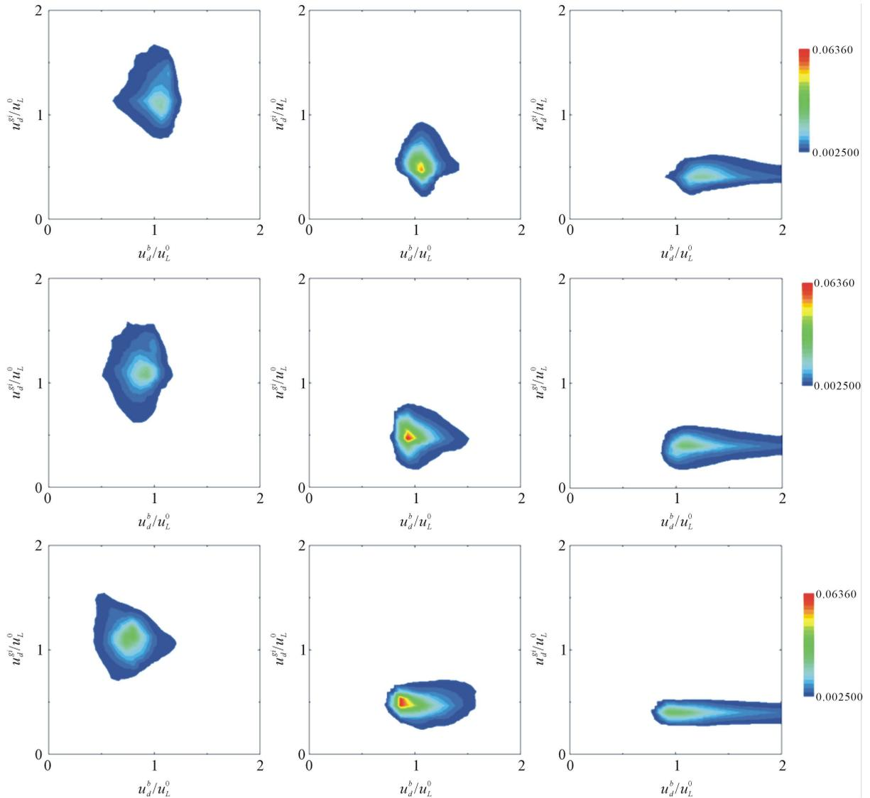
**Figure 4.** Joint pdfs between non-dimensionalised  $u_d^{gi}$  and  $u_d^b$  on some isosurfaces of  $c_T$  with different Lewis numbers. From the top, case Ml, case Mm, and case Mh, and from the left,  $c_T = 0.167, 0.690, 0.900$ .
