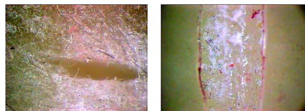
**Figure 15. Pictures of air bubbles entrapped in specimens.**
