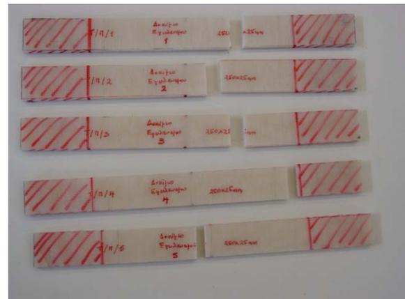
Figure 8. Failure mode of plate coupons in tension.
