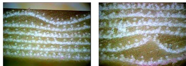
**Figure 16. Local misalignment of cotton textile layers.**
