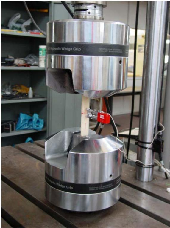
Figure 6. Tensile testing setup.
