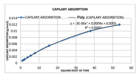
**Figure 2.** Capillary absorption vs  $\sqrt{t}$ .
