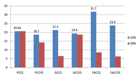
Figure 1. Shows the compressive strength at age 7 days for (Null, 10%, 20%) additive materials.
