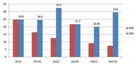
Figure 2. Shows the compressive strength at age 28 days for (Null, 10%, 20%) additive materials.
