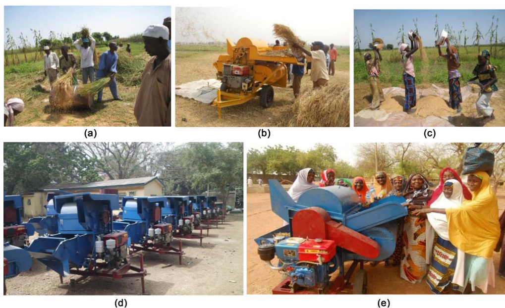
Figure 4. (a) Threshing paddy on drum, (b) motorized rice thresher/cleaner, (c) young girl winnowing threshed paddy manually, (d) thresher/cleaner manufacture by local artisan, (e) small thresher/cleaner adopted by women group to improve threshing and cleaning of paddy.
