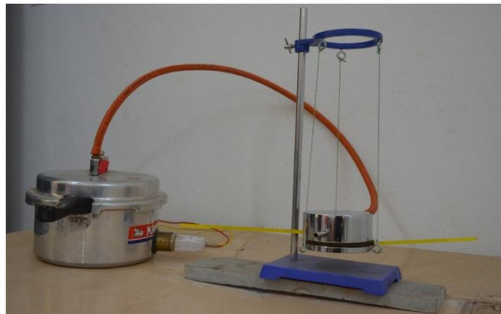
**Figure 2.** Experimental set up of Lee's disc Apparatus.
