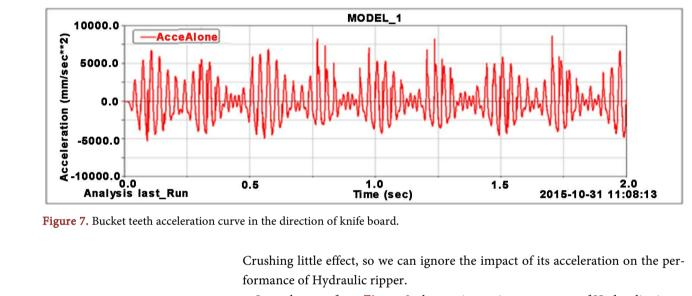
Figure 7. Bucket teeth acceleration curve in the direction of knife board.
