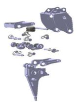
Figure 1. Hydraulic ripper explosion map.
