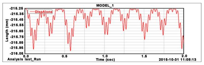
Figure 5. Bucket teeth displacement curve in the direction of knife board.
