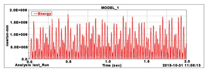
Figure 8. Hydraulic ripper impact energy curve.
