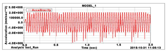
Figure 6. Bucket teeth acceleration curve in the direction of gravity.
