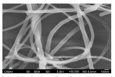
**Figure 2.** High resolution Scanning Electron Microscopy (SEM) micrograph to identify the topographic distribution of MWCNTs (0.05 mg/dl in SRS) applied on a glass coverslip. Magnification ×50,000, scale bar 100 nm.
