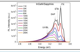
Figure 3. PL spectra as a function of sample temperature for an InGaN sample grown on sapphire by MBE.
