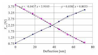
Figure 13. Linear ranges of the inverter cascades characteristics in configuration T + L and L + T; sensitivity T + Lwas 43.7 mV/nm and L + T was 38.2 mV/nm.
