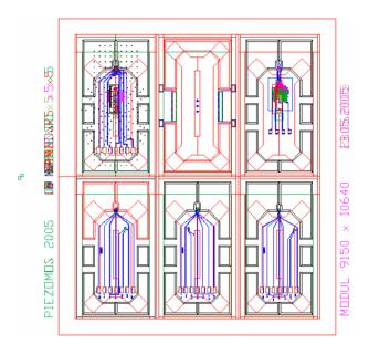
Figure 1. Layout of the six different chips of microprobes.
