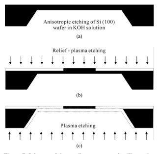
Figure 7. Schemes of the cantilever cross section illustrating relief technique, which was applied to form cantilevers of appropriate thickness.
