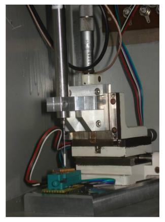
Figure 10. System for microprobe testing station - view inside the Faraday cage.
