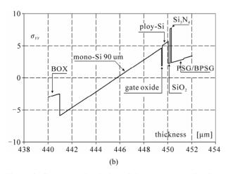
Figure 9. Computer simulation of the stress  $(\sigma_{YY})$  distribution over the cantilever upper surface (a) and graph across the cantilever thickness in the region of the MOS transistor gate (b); simulations were done with force 0.1 G concentrated at the cantilever tip, as well as with real layout and technology of the microprobe.
