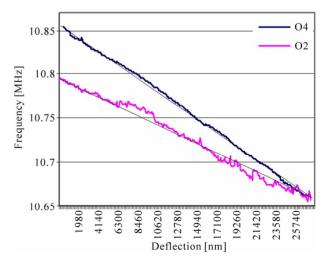
Figure 14. Frequency v. deflection characteristics obtained from measurements of microprobes O4 and O2. Sensitivities are 8 Hz/nm (the highest in the batch) and 5 Hz/nm (the lowest in the batch).
