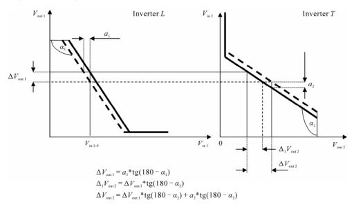
Figure 5. Amplification effect of the inverters cascade arrangement.
