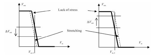
Figure 4. Switching characteristics of the inverters  $P_L + N_L$  and  $P_T + N$ , without and with stress.
