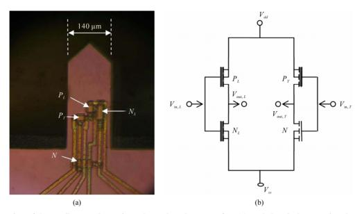
Figure 3. Top view of the cantilever and transistors located on the top surface (a), and electrical connections between transistors (b).
