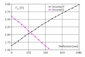
Figure 12. Comparison of extracted linear parts of characteristics Vout in function of the cantilever tip deflection for inverters T type and L type.
