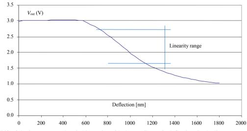
Figure 11. Shift of the inverter type L switching point with the cantilever tip deflection. In the linear part of characteristic measured microprobe sensitivity was -2.6 mV/nm.
