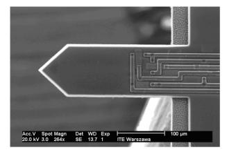
Figure 8. SEM top view of the silicon cantilever 2.87  $\mu$ m thick.
