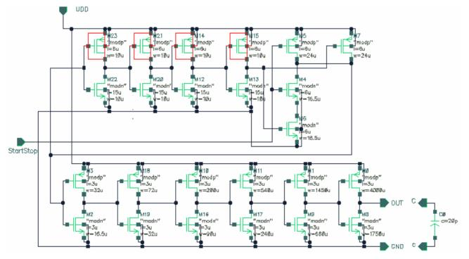
Figure 2. Diagram of the ring oscillator. White rectangles indicate transistors, which are located in the stressed area on the cantilever.
