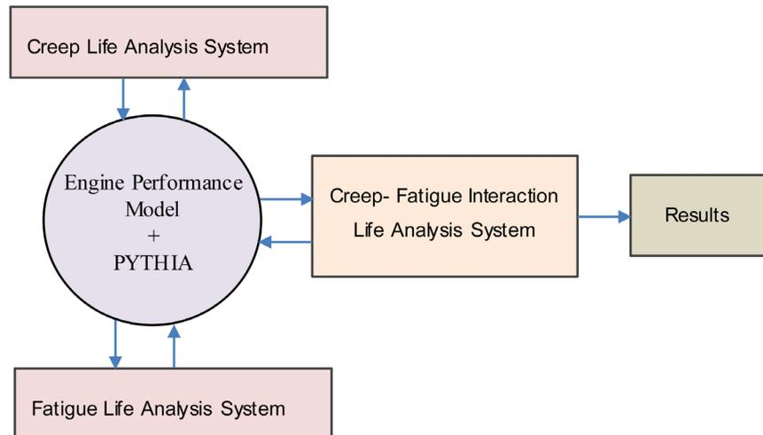
**Figure 1.** Creep-fatigue interaction analysis system.
