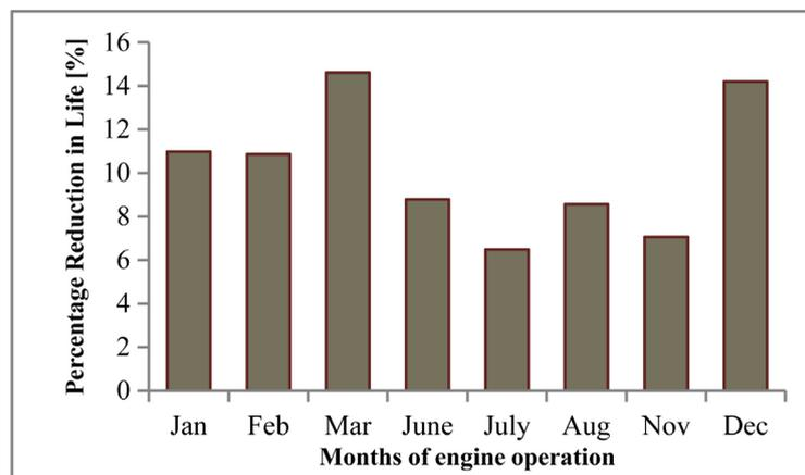
**Figure 5.** Percentage reduction in life due to fatigue interaction with creep.
