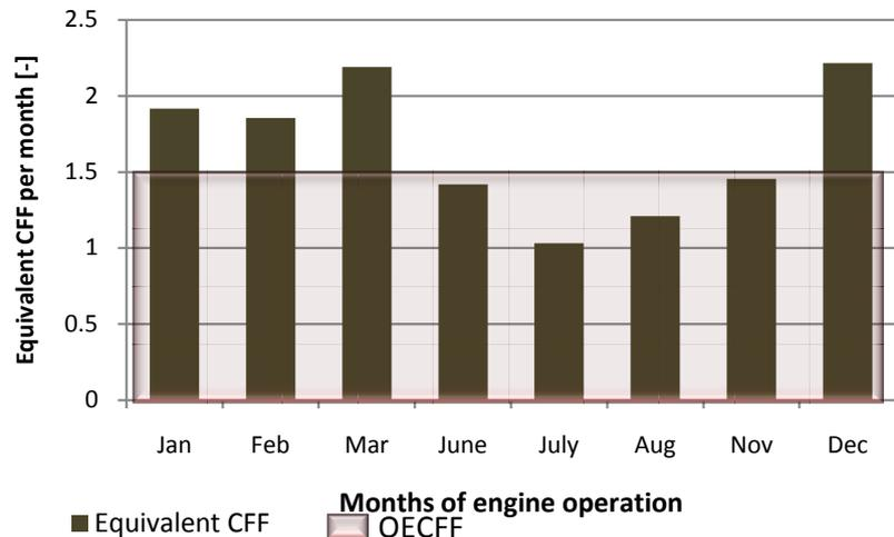
**Figure 3.** Equivalent creep-fatigue factors for each month of engine operation.
