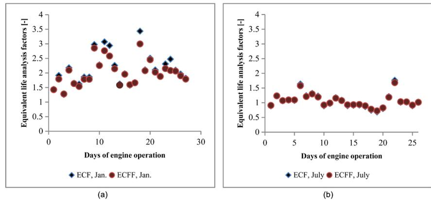
**Figure 4.** Comparison of equivalent creep factors and equivalent creep-fatigue factors in two months of engine operation.
