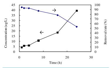
Figure 2. Effluent TP concentration and removal rate of PAC + AAL process.
