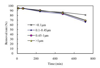
**Figure 6.** Removal rate of various size particulate phosphorus of PFS + AAL.
