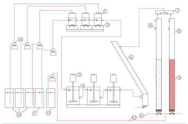
Figure 1. Sketch of the experimental device. Note: 1—raw water tank; 2—mixing cup; 3—magnetic stirring bar apparatus; 4—reacting cup; 5—stirring machine; 6—sedimentation tube; 7—distribution groove; 8—filtration column; 9—filter media; 10—overflow pipe; 11—effluent pipe; 12—backwash pipe; 13—backwash tank; 14—coagulation dissolving tank; 15—di-aphragm pump.
