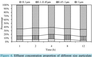
Pigure 4. Effluent concentration proportion of different size particulate phosphorus.
