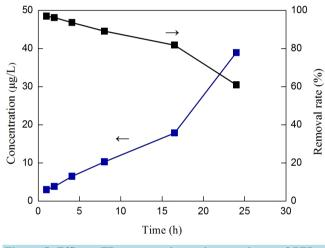
Figure 5. Effluent TP concentration and removal rate of PFS + AAL process.
