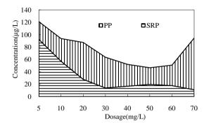
Figure 2. Concentration comparison of various forms of phosphorus by different dosage of AlCl<sub>3</sub>.
