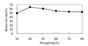
Figure 3. TP removal efficiency with different dosage of AS.
