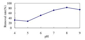
**Figure 8.** TP removal efficiency with different pH value of PAC.
