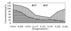
Figure 7. Effluent various forms of phosphrous concentration with different dosage of PAC.
