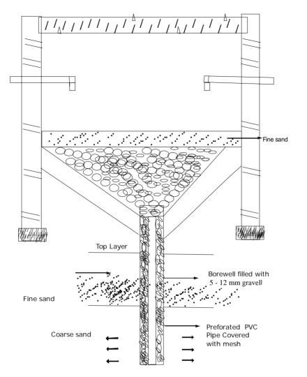
Figure 3. Schematic of recharge arrangement with a bore well.
