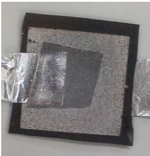
Figure 1. A photograph of sample D where Al was vacuum evaporated on the surface about 90% in area.
