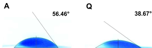
Figure 3. Images of water droplets and measured contact angle of an area unaffected by pollution (A) and a surface treated with the laser in Q-switch regime (Q).
