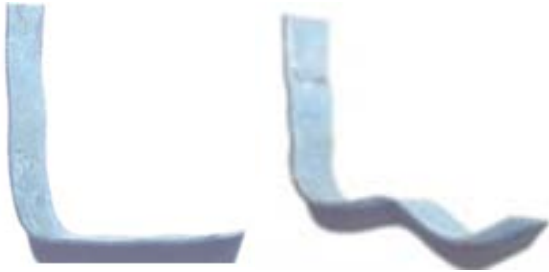
Figure 3. The Ni-Ti memory alloy films before and after deformation.
