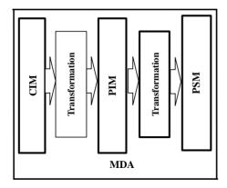
Figure 1. Model Driven Architecture.
