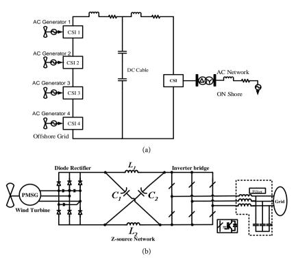
Figure 4. (a) CSI for offshore wind energy; (b) ZSI for wind energy.
