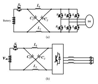
Figure 5. (a) ZSI for HEV; (b) ZSI for PHEV.
