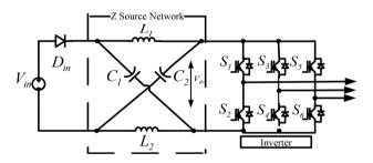
Figure 1. Basic topology of Z-source inverter.
