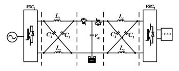
Figure 8. UPS system with Z-source network.
