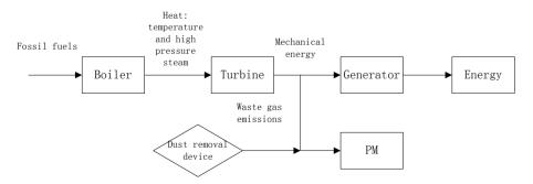
Figure 5. The respirable particulate matter emission principle.
