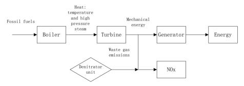
Figure 4. Nitrogen oxides emission principle.
