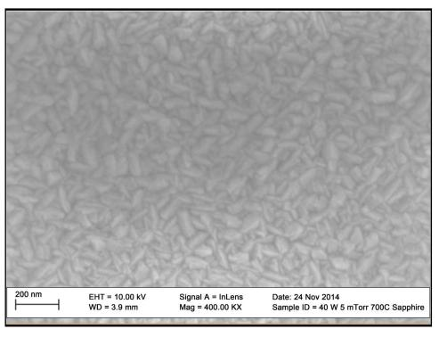
**Figure 6.** SEM surface images of sputtered GaN thin films. 40 RF power and 5 mT pressure using 700°C substrate temperature, grain sizes of 62 nm - 39 nm on sapphire wafer.
