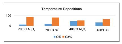
**Figure 7.** Bar graphs depicting the atomic percentage of oxygen vs gallium; Atomic percentage of oxygen vs gallium using temperatures of 400°C and 700°C on Si and Al<sub>2</sub>O<sub>3</sub> wafers.
