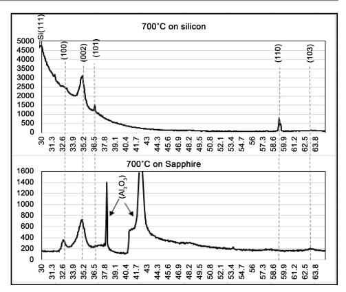
**Figure 5.** X-ray diffraction patters of GaN films; 40 RF power, 5 mT pressure and 700°C temperature.
