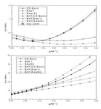
Figure 1. E/A in MeV for symmetric nuclear matter (upper panel) and pure neutron matter (lower panel) using different potentials at (T = 0) as a function of density using different potentials for continuous choice of the auxiliary potential.
