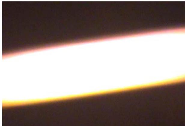
**Figure 2.** Horizontal spanned incandescent nichrome wire in air has different color on top (violet) and bottom (yellow) sides. Different glowing colors in space are varying along the gravity vector. The diameter of investigated nichrome wire is 1 mm. The length of spanned wire here is 20 mm. Camera SONY Digital Handycam DCR-TRV147E PAL Digital 8 with 560× digital zoom was used for the visualization.
