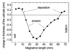
Figure 2. Structures of the target erosion.
