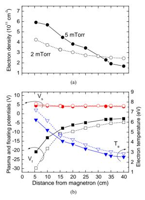
Figure 6. Axial distribution from the target exit of (a) Electron density  $N_e$ ; (b) Electron temperature  $T_e$ , plasma  $V_s$  and floating  $V_f$  potentials.  $I_{el.-magn} = 0$  A. Solid lines: p = 5 mTorr, I = 4 A, U = 323 V. Dot lines: p = 2 mTorr, I = 4 A, U = 370 V.
