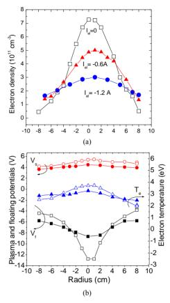
Figure 4. Radial profiles of: (a) The electron density  $N_e$ ; (b) Electron temperature  $T_e$ , floating  $V_f$  and plasma  $V_s$  potentials. 20 cm from the target. p = 10 mTorr, 50 sccm, W = 3 kWatt. Open symbols:  $I_{el} = 0$  A, solid symbols:  $I_{el} = -0.6$  A.
