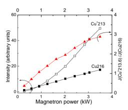
Figure 9. The optical emission intensities from Cu ion lines (213.6 nm) and Cu neutral (216.5 nm) at 10 mTorr vs discharge power.
