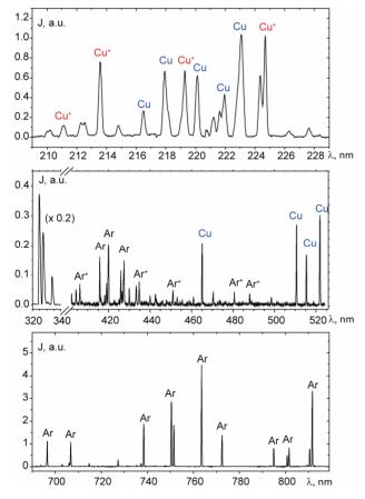
Figure 8. An optical emission spectrum from Ar/Cu plasma at wavelength between 210 and 830 nm. p = 5 mTorr,  $I_{el-mag} = -0.4$  A, W = 3.36 kW.
