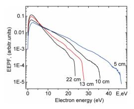
Figure 7. Normalized electron energy probability function on the discharge axis. p = 5 mTorr, W = 1.3 kWatt.
