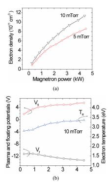
Figure 5. (a) Electron density; (b) Plasma potential  $V_s$ , floating potential  $V_f$ , and mean electron temperature  $T_e$ ; as function of the magnetron power.  $I_{el} = -0.6$  A. 20 cm from the target.
