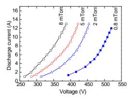
Figure 3. Current-voltage characteristics of the HCM for various pressures.
