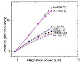
Figure 10. Normalized intensities of Ar and Cu spectral lines as function of a magnetron power,  $I_{el} = -0.5$  A, 10 mTorr.
