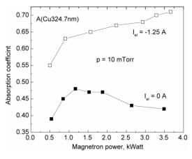
Figure 11. Absorption coefficient A of the Cu spectral line 324.7 nm as function of magnetron power.
