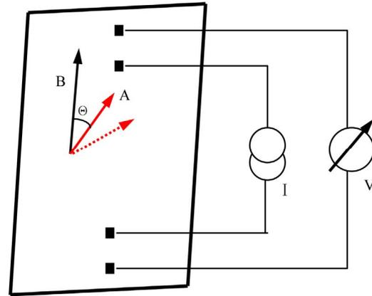
**Figure 1.** A schematic of the measurement of AMR for different angles, where the direction of cooling field is represented by the black arrow B, and the direction of applied external field is represented by the red arrow A.
