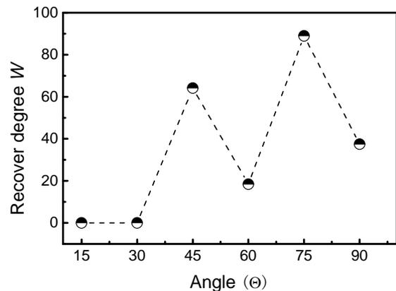
**Figure 5.** The recover degree  $W$  of normalized AMR dependent on the angle which formed with respect to cooling field direction. The horizontal axis corresponds to the angle  $\Theta$  between external field and cooling field.
