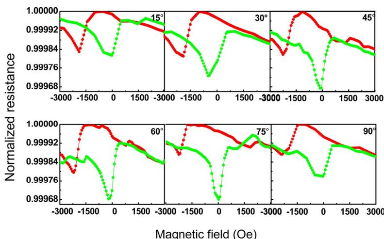
**Figure 3.** The recover degree of normalized AMR peaks value along the cooling field after performing a external perturbation field which forms certain angle  $\Theta$  with respect to cooling field direction,  $\Theta$  is 15°, 30°, 45°, 60°, 75°, and 90°, respectively.
