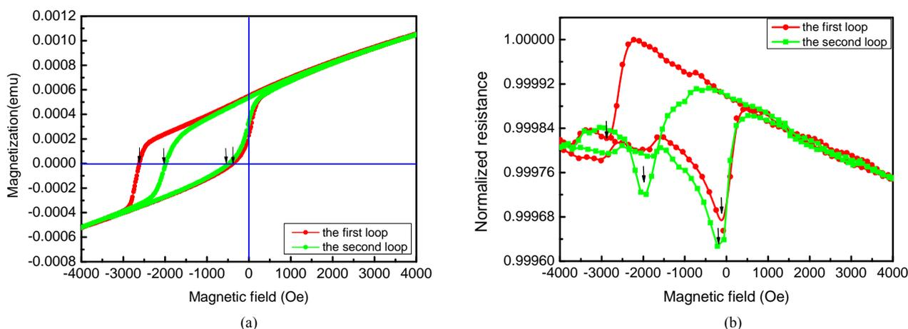
**Figure 2.** The hysteresis loops in 10 K (a) after the sample was cooled in the field of 4000 Oe. The normalized AMR loops was also measured in 10 K. The arrows indicate that the coercivity field in is corresponding with the normalized AMR peaks value, respectively.
