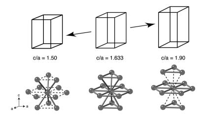
**Figure 1.** Hcp structures with three different *c/a* axial ratios. The top figures show the hexagonal unit cells and the bottom figures show the atomic arrangement. The first nearest neighbors are connected by thick bonds while the second nearest neighbors are connected by broken lines.
