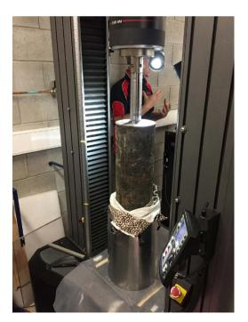
**Figure 1.** Bentonite plug under test using an Instron 250 kN electro-mechanical loading frame. A split collar was designed to sit against the top face of the cylinder loading seat to guarantee axial alignment of the casing with the test macine.
