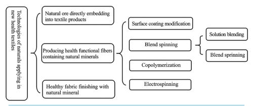
Figure 1. The flowchart of the processing methods of health textiles containing natural minerals.
