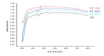
Figure 3. UV-Vis-NIR spectrum of sub-bituminous coal sample
