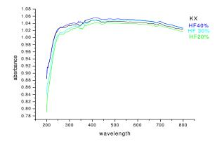
Figure 2. UV-Vis-NIR spectrum of bituminous coal
